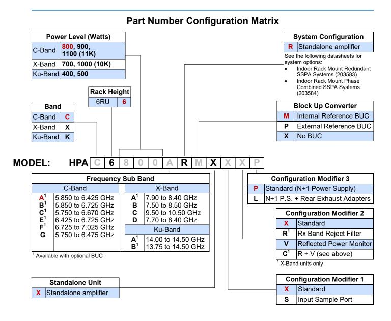
**Example** - A standalone 800W GaAs C-Band 6RU Rack Mount SSPA with standard N+1 external power supply and an optional internal reference block up converter is part number: **HPAC6800ARMXXXP**.
